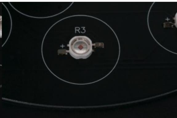
That leads to an important distinction: Multi-chip/quad-lens units mix colors together inside of the lens, whereas single-chip/lens fixtures mix colors outside of the lens. Color mixing within the lens results in more
